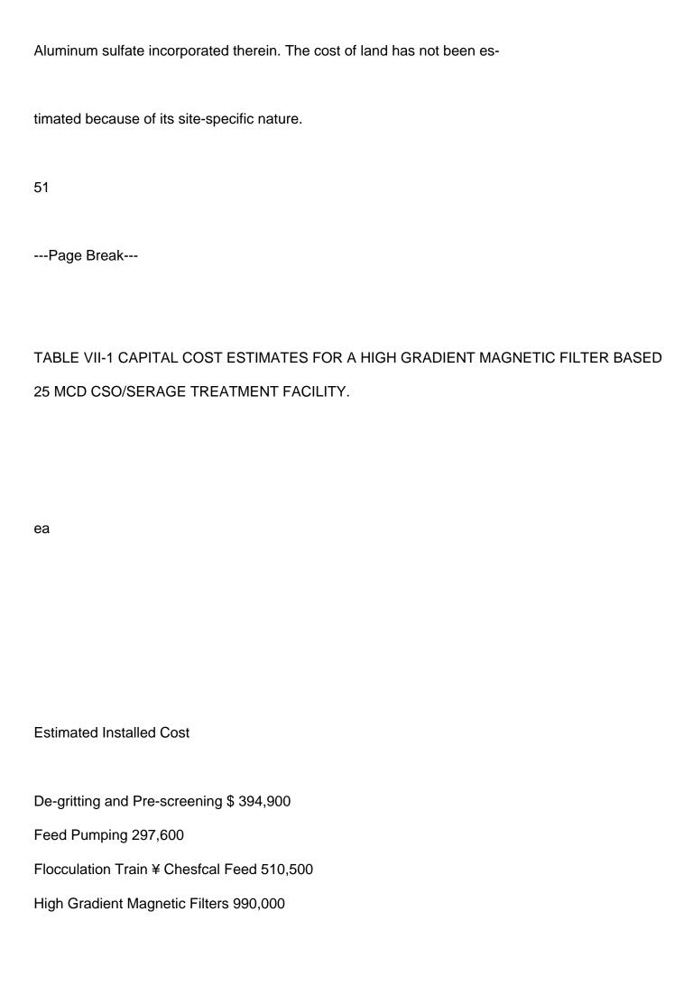
Back#lusing 441,300 Filter Piping and Valving 327,600 Thickening and Dewatering 265,600 Disinfection 86,900 Flectrical 337,100 ?Automatic Process Control & Monitoring 258,700 Physical Plant Construction 490,000 Subtotal: \$4,100,000 Construction Contingency 10% 410,000 Subtotal: \$4,500,000 Engineering and Adainistration 15% 677,000 TOTAL ESTIMATED CosTs: \$5,187,000 Pert 2
