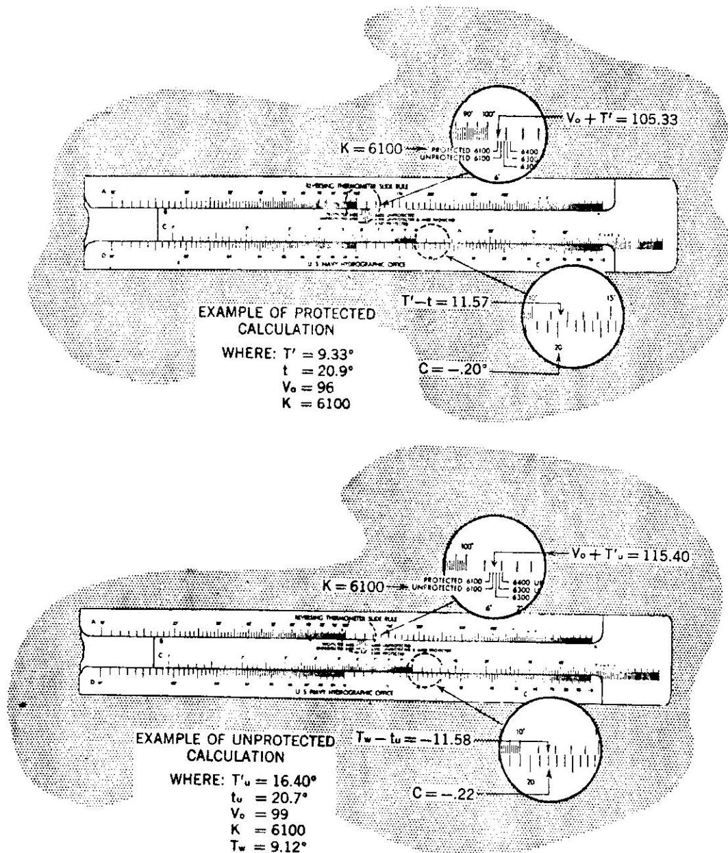
Figure 3-2. Two drawings of reversing thermometer slide rule with protected and unprotected sample calculations.
